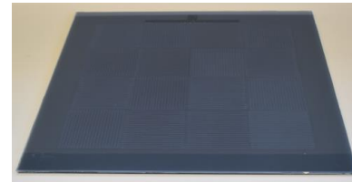
Busbarless TOPcon + imec's TWILL technology
