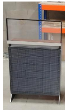
BIPV curtain wall demo
