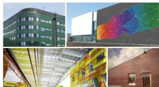
Building-integrated PV (BIPV)
